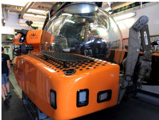
Fig. 1. Triton 7K3 submersible, Aurelia showing the Titan 4 hydraulic arm, the prime tool used for sampling deep-sea organisms during the expedition.
