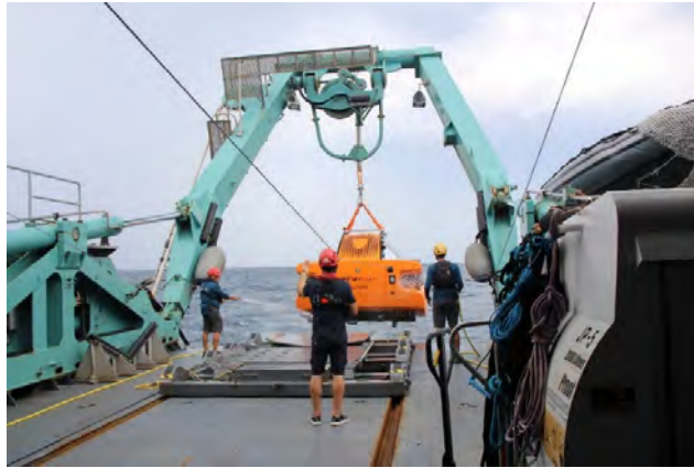
Figure 3. Recovery of Triton 7K3 Aurelia from the stern of the Odyssey. Note the tugger lines on either side and the tow line attached to the back of the submersible.
